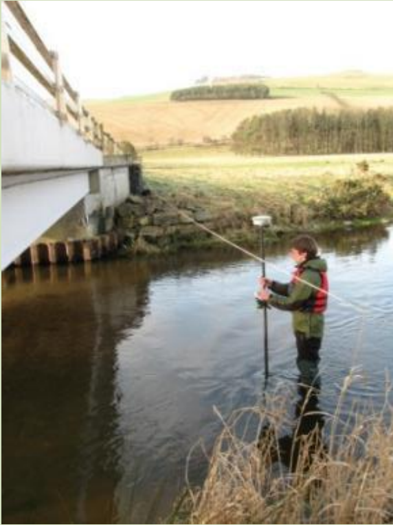
Photo 4: Surveying river morphology on Bowmont Water near Town Yetholm
