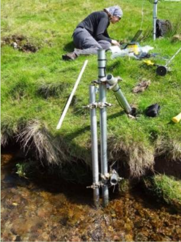
Photo 6: Downloading data from a flow monitoring station on a headwater tributary of Bowmont Water
