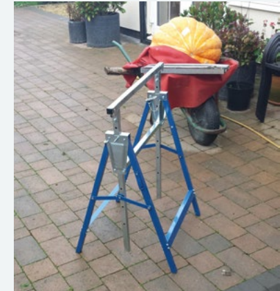
Figure 3 Carpenters' telescopic trestles used to support a heavy sofa above flood level
