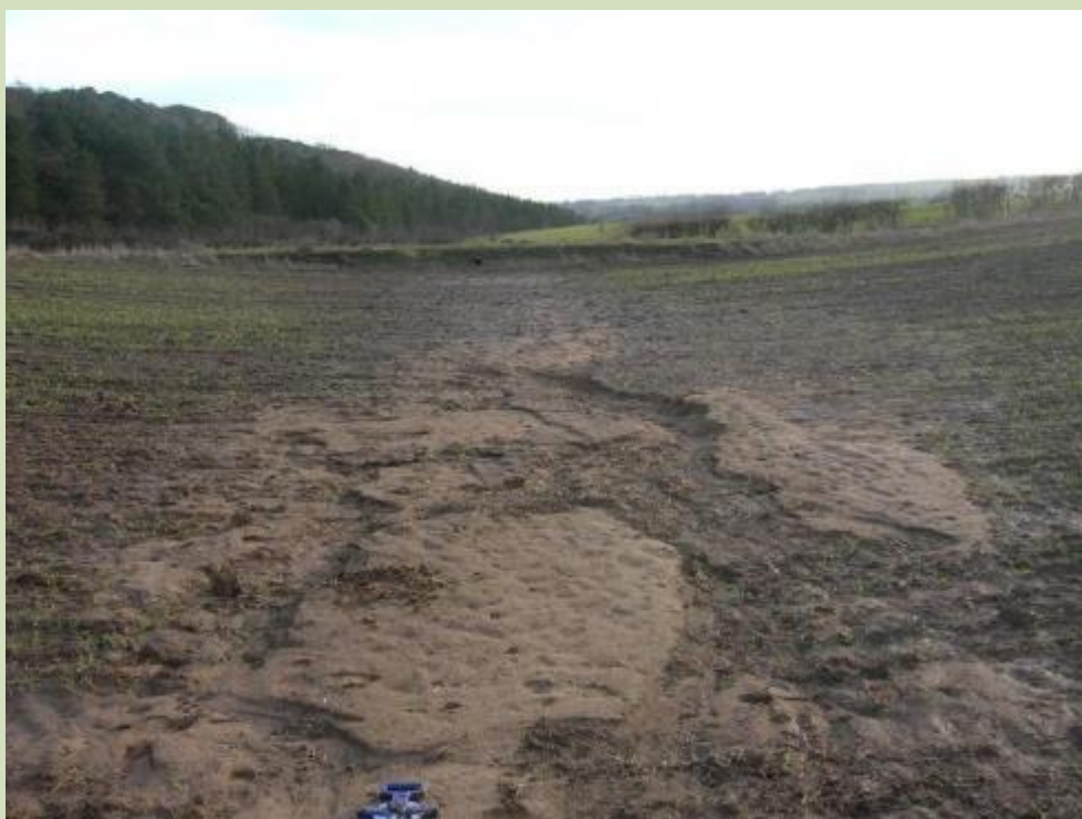
Figure 12: Sediment captured in overland flow RAF. Approximately one tonne of sediment was captured in a single event in January 2010.
